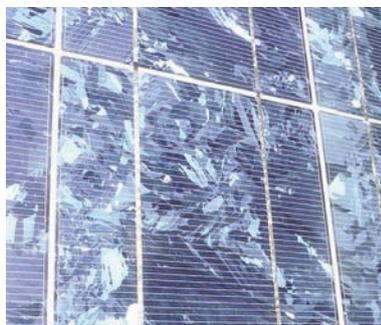
Figure 2: Cellule de silicium polycristallin
